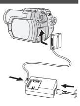
While the DC cable is connected to the AC adaptor, the battery will not charge.
